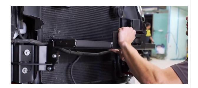
24. Lift winch cradle onto sub supports and secure with M10x30 bolts, flat washers and flange nuts
