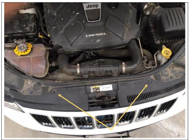
3. Next step is to remove the rest of the front bumper. Start with bonnet/hood open and pry out two clips shown with trim tool or flat head screw driver.
