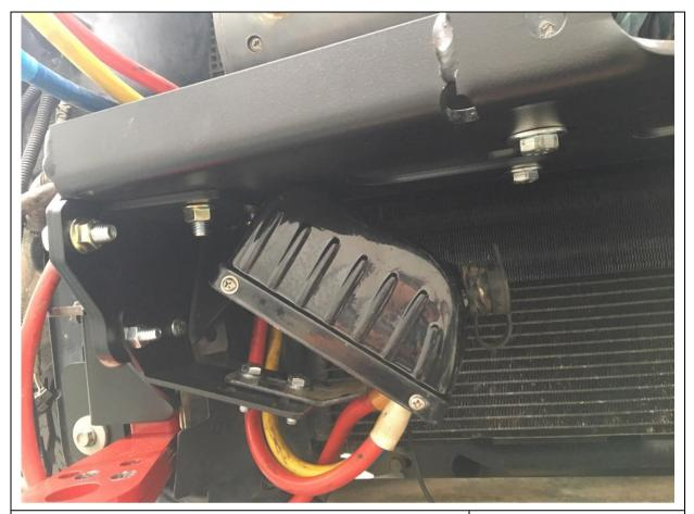
27. If you are fitting a winch that does not have an integrated control box (like a Warn Zeon) then you can use the supplied winch controller bracket to mount your control box as shown. Use one existing M10 bolt and then add M6 bolt washer and flange nut.
