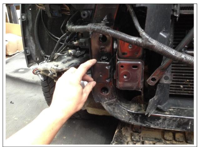
19. Cut tab off shown in picture from both sides.
