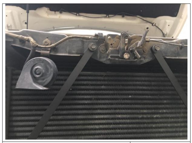
25. Fit radiator braces as shown with factory bolts.
