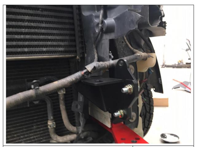
22. Fit sub support with M10 bolts, flat washer and flange nuts.
