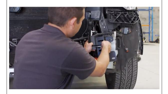
20. Place mount on chassis and fit reusing factory M8 bolts.
