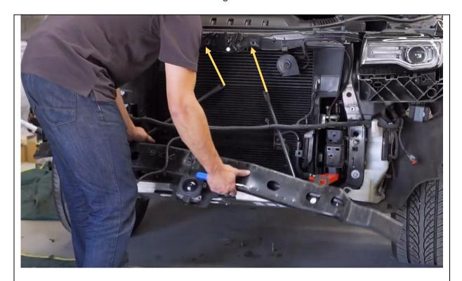
16. Remove 2x screws with 13mm tool holding round support bars from top of bonnet support then remove entire reinforcement bar.
