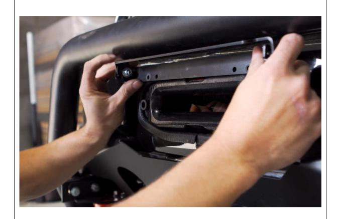
39. If purchased, fit number plate flip to bumper. Drill holes and fit with M6 supplier hardware from number plate flip
