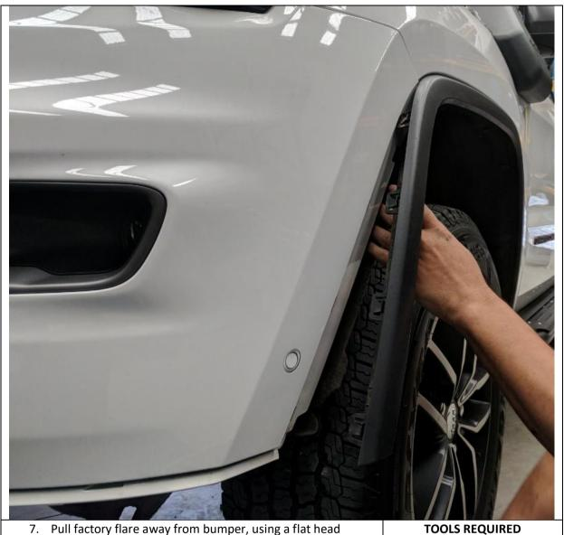
7. Pull factory flare away from bumper, using a flat head screwdriver release at least 2 of the push in clips on top edge being careful not to break them as you pull the flare away from the body.
