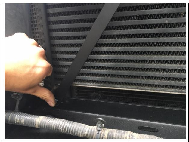
26. Fit lower end of radiator supports to winch cradle with M6 bolts, flat washers and flange nuts.
