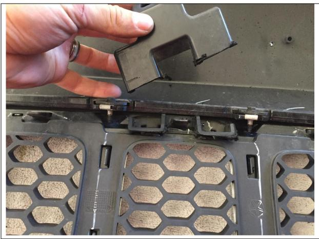
30. Some winches are larger than others and require you to cut off plastic protrusion inside the bumper, as shown above
