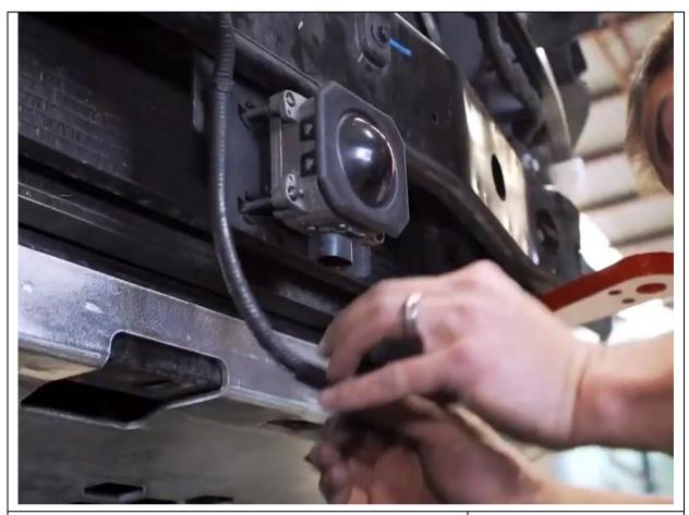
15. If Adaptive cruise control is fitted, unplug loom and pull sensor off posts.
