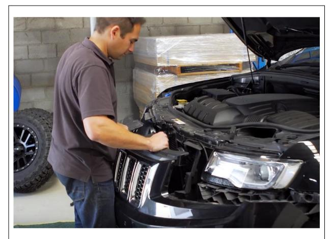
9. Lifting the top section ever so slightly you can release clips holding in the top section and pull the remainder of the bumper away.
